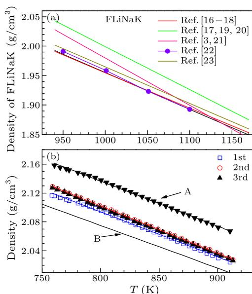
**Fig. 4.** (a) Density of FLiNaK measured by different researchers.<sup>[4,16-23]</sup> (b) Temperature dependence of FLiNaK density measured. The 1st, 2nd, 3rd are the three separate runs of measurements. Curve A is the density by averaging the results of three runs taking into account of the surface tension, and curve B is the density calculated by additive principle.
