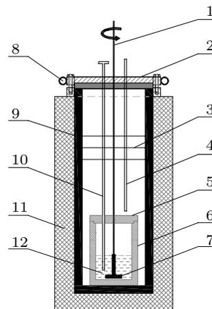
**Fig. 2.** Schematic diagram of the cooling curves measuring device: (1) stainless steel connecting rod, (2) brass lid, (3) heat insulation plate, (4) corundum inlet pipe for Ar gas, (5) BN crucible lid, (6) BN or graphite crucible, (7) graphite stirrer, (8) copper cooling pipe, (9) corundum furnace tube, (10) thermocouple, (11) thermal insulator, (12) molten salts.
